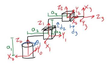
5. Shown here is a labeled kinematic diagram. Find the complete homogeneous transformation matrix (HTM) from the base-frame to the end-effector frame by first finding the rotation matrices and the displacement vectors, then assembling into the HTM.
