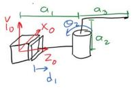
8. (Graduates Only): Shown here is the kinematic diagram of a 3-degree-of-freedom manipulator. Find the inverse kinematics equations.
