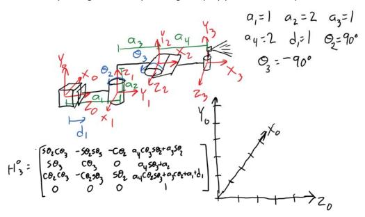
8. (Undergraduates Only): Shown here is the kinematic diagram of a 2-degree-of-freedom manipulator. Find the inverse kinematics equations.
